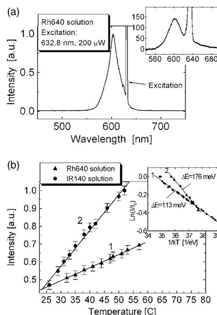
FIG. 1. (a) ASL spectrum of Rhodamine 640 solution and Rhodamine 640 dye encapsulated in 35 nm silica shells (inset); (b) temperature dependence of ASL for Rh640 solution (●) (excitation—He–Ne laser,  $\lambda=633$  nm) and IR-140 solution (▲) (excitation—Nd:YAG laser,  $\lambda=1064$  nm). The activation energy estimated for each dye is shown in the figure inset and this calibration is used for temperature mapping under confocal microscope.
